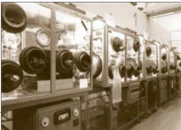
Glove compartments in the plutonium laboratories. A glove compartment is a gas tight cabinet, generally made from transparent plastic, in which operators can work on certain radioactive materials such as plutonium, using the gloves that reach into the cabinet.
