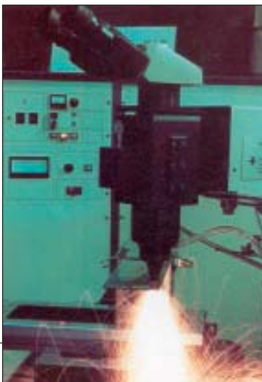
Laser research for cutting metals and treating surface coatings
